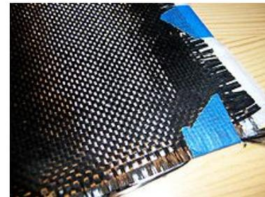
Fig 11: Carbon Fiber Cloth – commonly used in composite construction
