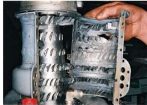
*Fig 3: Damage in a compressor case [5]*
