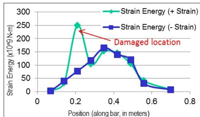
Fig. 15: Graph of strain-energy response; location of damage can be identified by the peaks [1]
