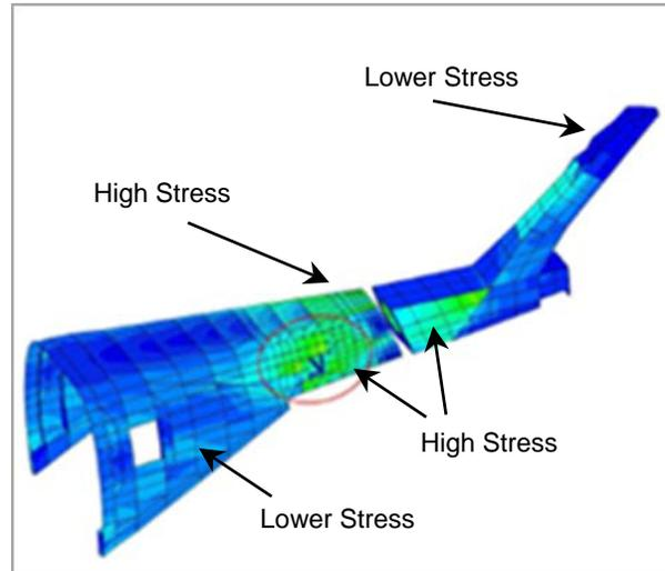
Fig. 9: FE Stress model of a tail section; hot spot analysis
