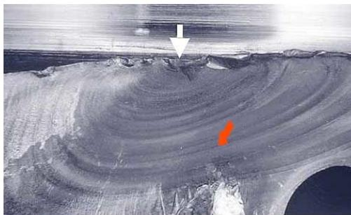
Fig 12: Fractured aircraft engine crankshaft. Beech Marks are a sign that a crack progressed across the part and failure was due to metal fatigue (red arrow). The white arrow shows the crack initiation point. [7]
