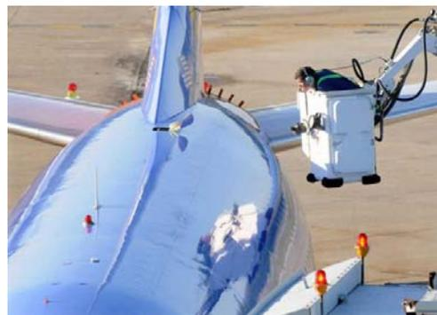
*Fig. 4 shows the Southwest Airlines airplane where in 2011, a hole occurred in-flight on the roof of the aircraft while cruising at 35,000 feet. Federal investigators and National Transportation Safety Board (NTSB) determined metal fatigue as the cause: a crack developed in an area where two sheets of aluminum skin were bonded together.*
