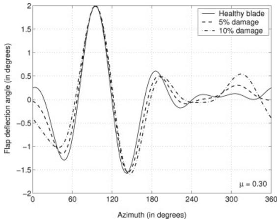
Fig. 5: Optimal Flap Control Input for a Healthy versus a Damaged Rotor Blade,  $\mu=0.30$  [6]
