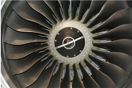
*Fig 2: The leading edges on first stage rotor blades often have damage from foreign objects that is difficult to visualize*
