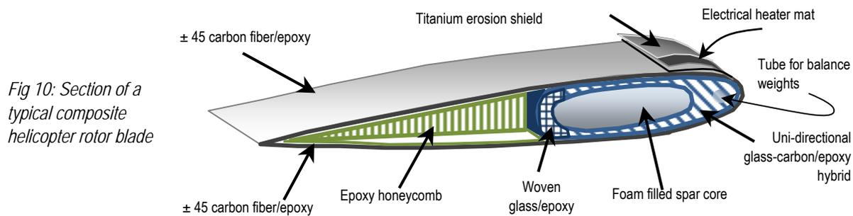
Fig 10: Section of a typical composite helicopter rotor blade
